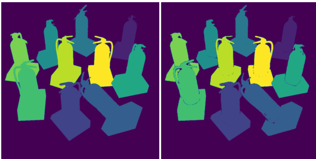
Figure 9: Clean segmentation map(Left) and noisy segmentation map(right) . The right segmentation map is generated by pre-trained model and without post-processing.
